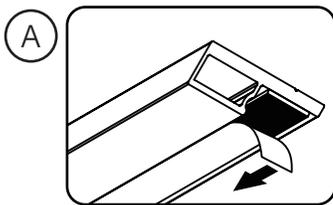
**A** Apply double sided tape and remove the protective film.
