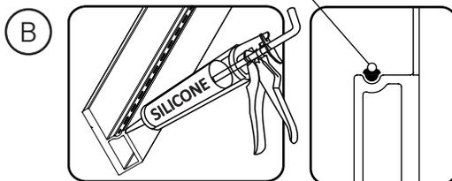
**B** Put silicone in the groove, on the full length of the flange.
